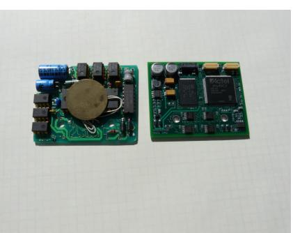
Figure 1 - Old and new CPU board
